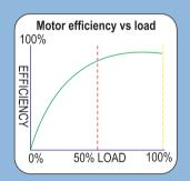
Due to motor torque being proportional to the square of the applied voltage it is possible to reduce the applied voltage, to match the motor torque to the load torque, according to the job of work that the motor is doing at any point in the duty cycle. Reducing the voltage reduces apparent power (kVA), active power (kW) and reactive power (kVAr). The illustration on the left shows the relationship between kVA, kW and kVAr.
